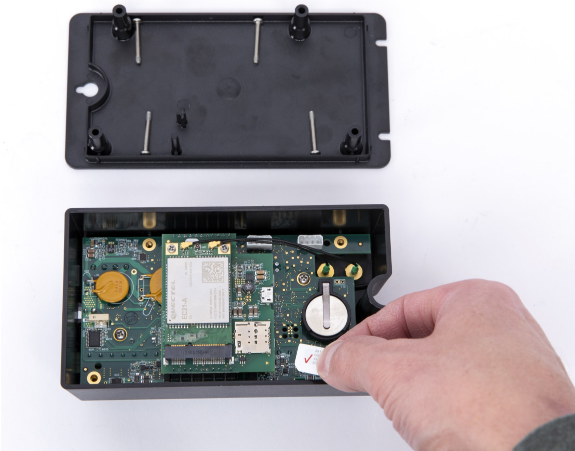
FIGURE 11-1. SIM card installation
